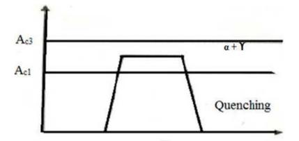
Heat treatment path for intercritical annealing
